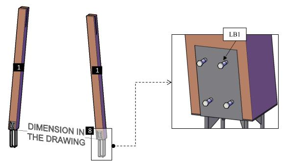
**Step 2:** Attach the single supports-A (2) to the posts with 3/8" x 7  $\frac{1}{4}$ " bolts (BL1). Each part has a series of numbers that indicate where to attach the part with the corresponding number.
