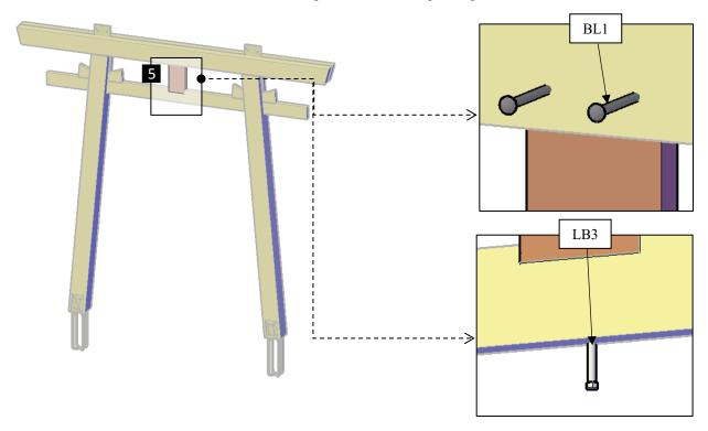
**Step 7:** Finally, Attach the simple support-C **(4)** to the metal plaques **(8)** with 3/8" x 9 ½" bolts **(BL3).** Each part has a series of numbers that indicate where to attach the part with the corresponding number.
