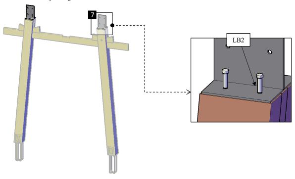
**Step 5:** Attach the simple support-B (3) to the metal plaques (8) with 3/8" x 8" bolts (BL2). Each part has a series of numbers that indicate where to attach the part with the corresponding number.
