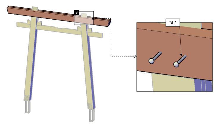
**Step 6:** Attach the reinforcement of support **(5)** to the supports with 3/8" x 6" lag bolts **(LB3)** and 3/8" x 7 1/4" bolts **(BL1).** Each part has a series of numbers that indicate where to attach the part with the corresponding number.
