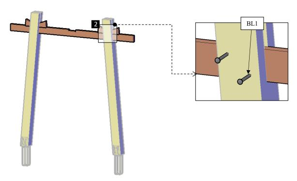
**Step 3:** Attach the molding **(6)** to the post with 3" deck screws **(DS1).** Each part has a series of numbers that indicate where to attach the part with the corresponding number.
